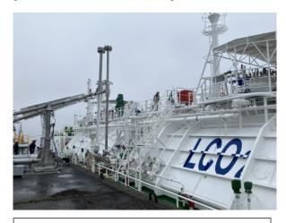
${\boldsymbol \cdot}$  "EXCOOL" berthing at onshore terminal Liquefied  ${\rm CO}_2$  is being transferred through the loading arm shown in the middle.
